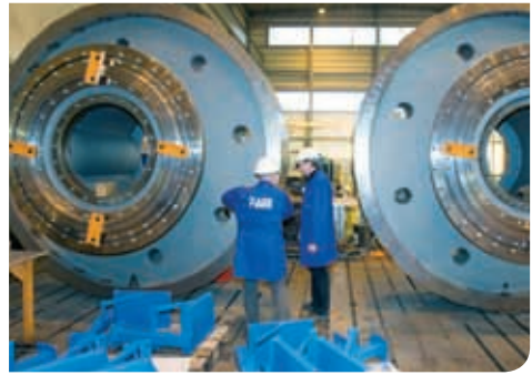
Rotors on a direct drive for bucket-chain excavators at FAM in Magdeburg
